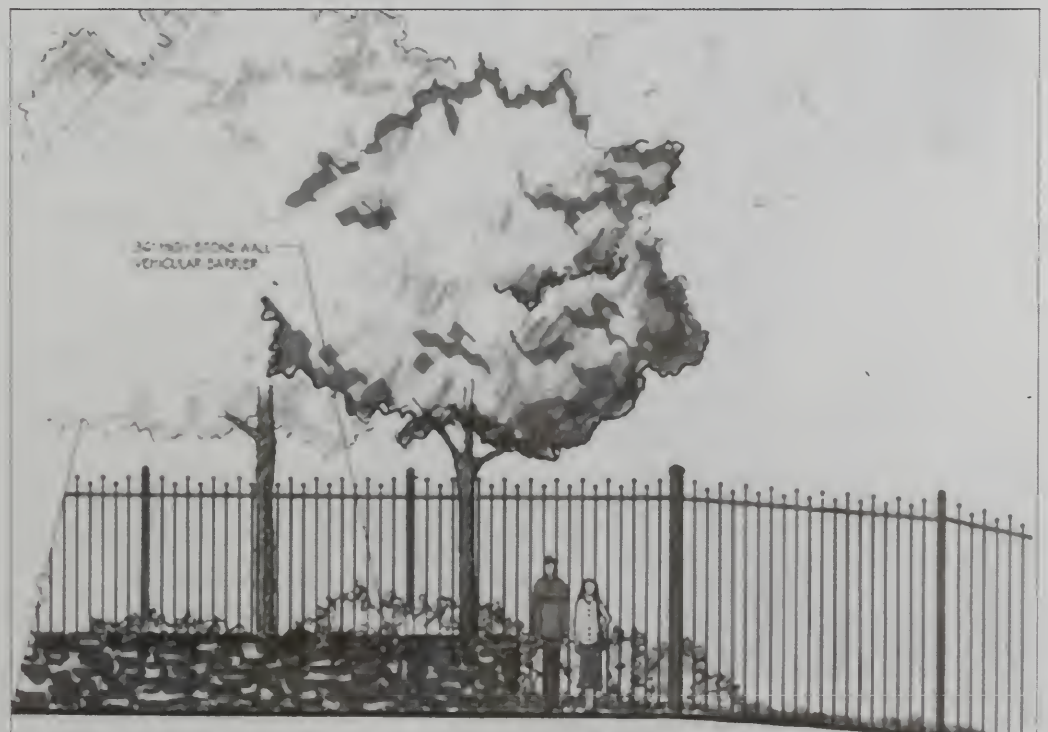
A 3-foot high stone wall will be built to prevent vehicle entry.
