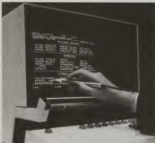
MIS video display terminals used a light pen to select information.
