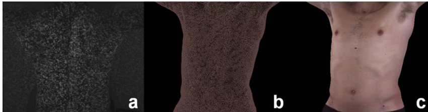
The camera pods used in stereophotogrammetry contain black and white cameras to help build a 3-D image (image a), a projector that displays a complex speckled pattern on the person's body surface which is read by a software program to create the image (image b) and a color camera to provide surface tone (image c).
